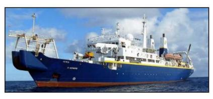
The IT Intrepid is a fully furnished cable ship capable of installation and maintenance activities in all ocean depths. Her immediate responsibility is to be on cable repair and maintenance stand-by for the Sentinel Maintenance program. The IT Intrepid is fitted with the IT ROVJET 207 for cable work and inspection to 2,600m.
